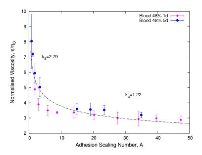
**Figure 6.** The figure shows the normalized viscosity of the blood samples against the Adhesion Number, A, correspondent to the non-Newtonian  $k_a(\dot{\gamma}_F, a) = 2.79$  an  $k_a(\dot{\gamma}_F, a) = 1.22$  for the Newtonian regime. We appreciate the collapse of the viscosity curves as a result of our scaling method.
